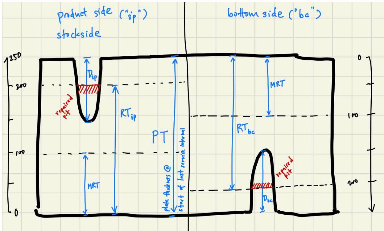
Figure 1 Diagram for CRA and LCR
