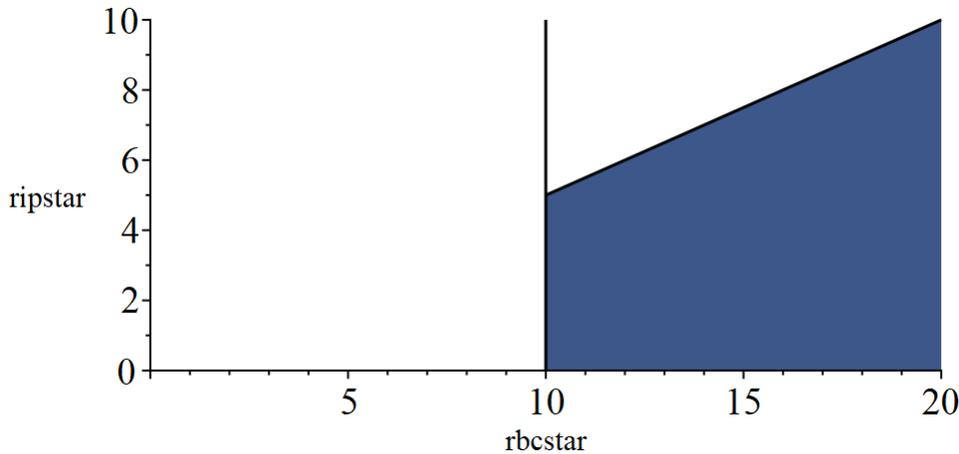
Figure 5 Bounding corrosion rates for bottom failure (shaded area is failure). Ripstar is LCR topside corrosion rate. Rbcstar is bottom side LCR corrosion rate. In this plot f ranges from 0 to 1 (unrealistic)
