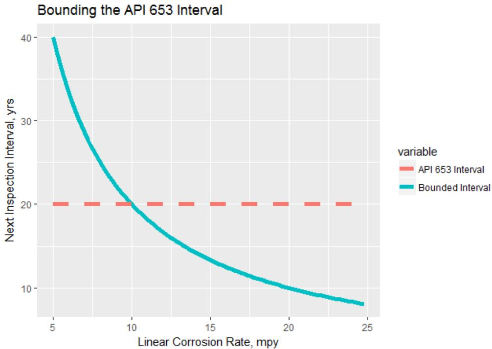
Figure 7: API and Bounding Corrosion Rate
