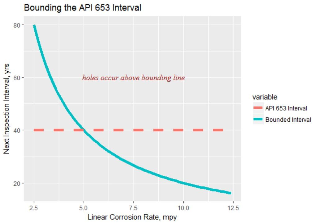
Figure 6: API and Bounding Corrosion Rate
