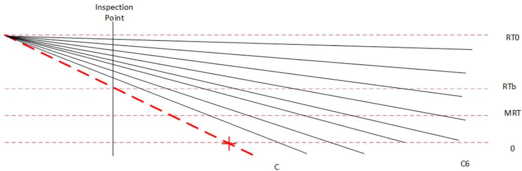
Figure 4: 1 Multiple API 653 Corrosion Rates Depend on  $RT_a$
