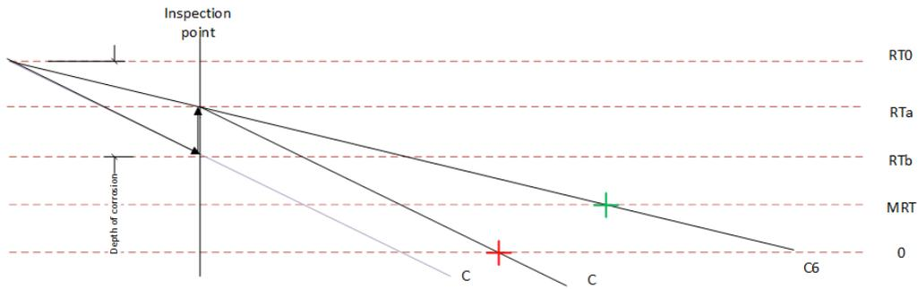
Figure 3: 1 Negative of line slope is corrosion rate
